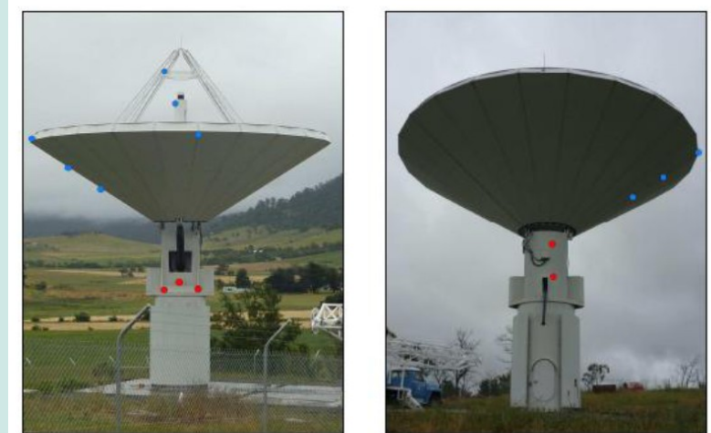
Fig 2: Target placement on front (left) and back (right) of the Hobart 12m telescope. The red circles are targets used to determine the azimuth axis, and the blue circles are targets used to determine the elevation axis.
