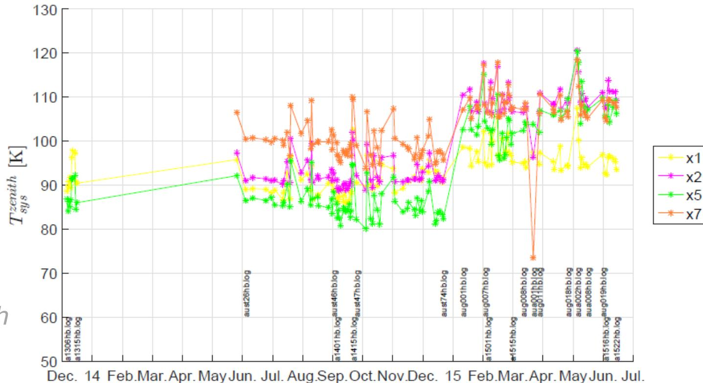
*X-band  $T_{sys}$  measurements of Hobart12 during the Austral experiments: jump coincides with recabelling event.*
