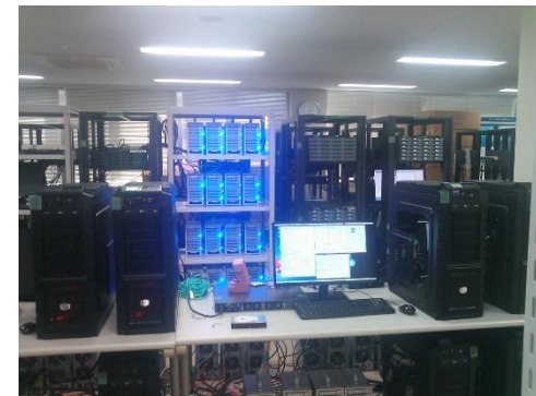
From 2015, the newly developed software correlator starts correlation operating in Mizusawa. Core engine of correlator is GICO3 developed by NICT.
