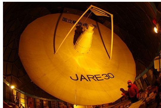
11m Multiple-purpose satellite receiving antenna in Syowa Station.
