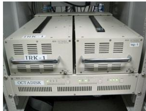
In 2014, the 1-Gbps recording system replaced to OCTADISK HDD data storage system. Recording time is 80 hours/unit.
